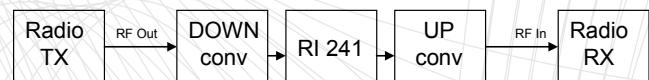
Fig. 2 If the IF interface is not accessible, RI 241 can be connected in the RF path using proper down- and up-converters.
